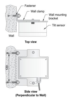
Figure 3: Installation perpendicular to the wall
