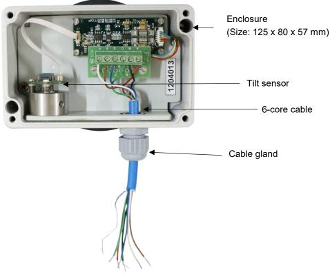
Figure 1: EAN-91M tilt meter
