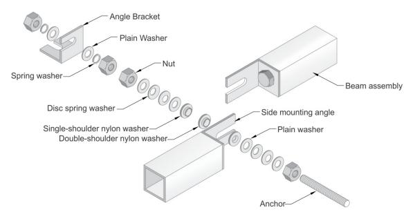
Figure 4: Installation of the anchor and the nuts & washer set
