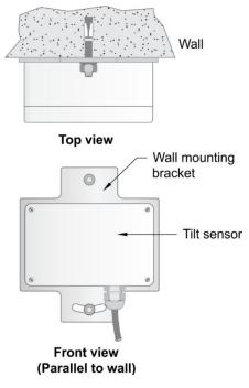
Figure 2: Installation parallel to the wall
