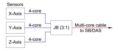
Figure 5 – Sensor connection to junction box
