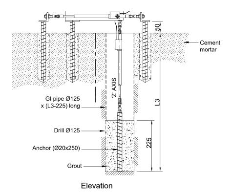
Figure 4 - Installation plan & elevation
