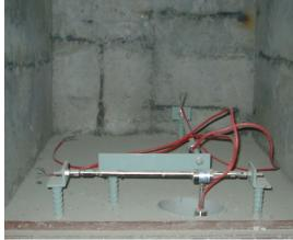
Figure 8 (a): Sensor connection with junction box – Z axis on top of the block
