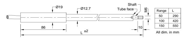
Figure 3-1 – vibrating wire sensor
