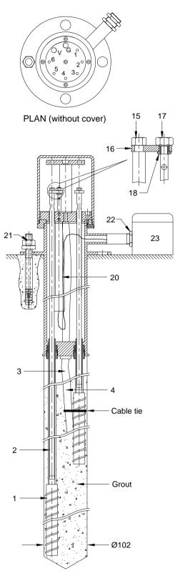
Figure 2.4 - Six point BHE detailed assembly
