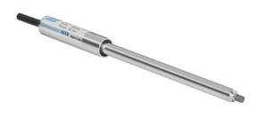
The retractable shaft of the sensor has a male thread of M6 x 12 to which the connecting rod can be attached through a link system. The sensor is provided with an integral 1 m long  $\phi$  4 mm four core cable with cores in red, black, green and white. Red and black cores are for frequency signal while green and white are for temperature monitoring through a thermistor.
