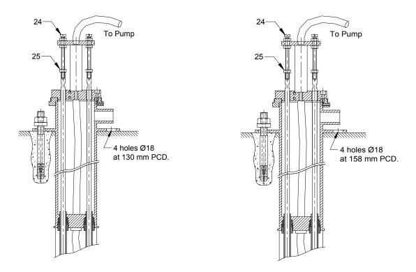
Figure 3.2 – Setting arrangement for 3pt BHE
