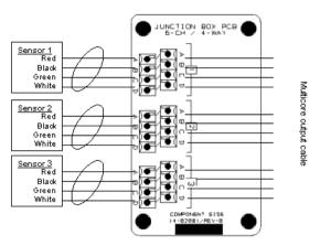
Figure 3.4 – Junction box wiring diagram
