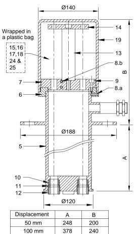
150 mm 510 300 Figure 2.3 - Six point BHE reference head assembly
