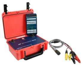
Fig 3.5 - Vibrating wire indicator
