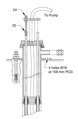
Figure 3.2 – Setting arrangement for 3 point BHE
