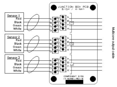
Figure 3.5 – Junction box wiring diagram
