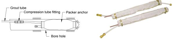
Packer anchor with geotextile bladder inflated with grout is generally used in fractured rock or soil.
