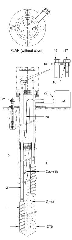
Figure 2.2 - Three point BHE detailed assembly
