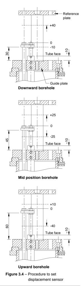
For any other required range, set distance 'C' accordingly. For example, when installing a BHE with 50 mm displacement in a vertically downward borehole, settlement is expected and setting range specified may be -10/+40 mm. In such a case connecting rod end distance from guide plate top (7) should be set at (45 -15) i.e. 30 mm.
