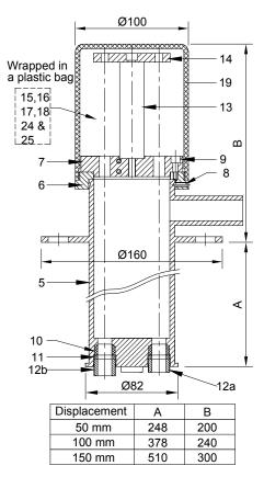
Figure 2.1 - Three point BHE reference head assembly
