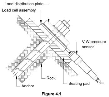
centralize it. If a bush is used, take care that it does not interfere with loading pattern of load cell. In case surface of flat seating pad and load distribution plates cannot be maintained parallel, use spherical settings or wedges or compensation washers made of copper/high density plastic material.
