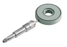
km without appreciable degradation caused by variation in cable resistance that may result from water penetration, temperature fluctuations, contact resistance or leakage to ground. The load cell is often used in series with a hydraulic jack for applying load. Consequently, it verifies load as applied by the hydraulic jack.
