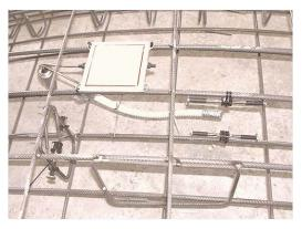
Figure 4.5: Stress cell installed with strain gages in concrete segments
