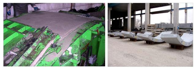
Figure 4.6: Concrete segments with stress cells and strain gages installed inside
