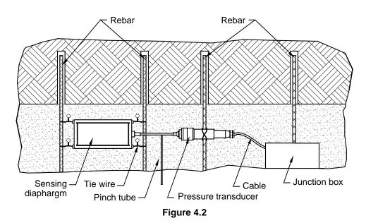
The flat rectangular capsule is firmly tied to the rebars by soft iron wire/cable ties using the four lugs provided. In case a reinforcing mesh is used, the flat rectangular capsule may be tied to this mesh. The cable is firmly fixed to another reinforced bar or reinforcing mesh and generally routed to a close by junction box. It is terminated here or later on joint to take the signal to a distant location.
