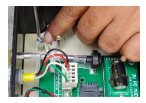
Figure 9-8: Fixing back the screw with Kevlar reinforcement
