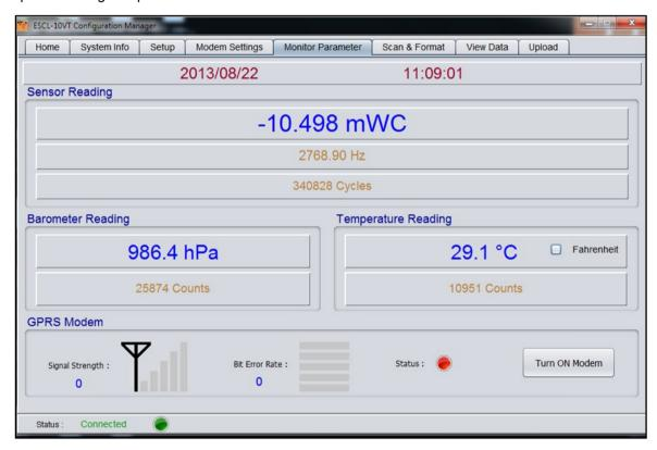
Figure 8-26: EWLR-101 Configuration manager – Monitor Parameter
