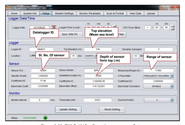
Figure 8-25: EWLR-101Configuration manager – Setup
