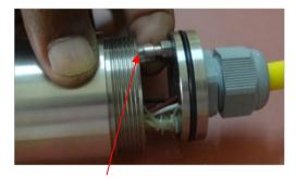
Figure 8-18: Connecting vent port
