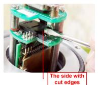
Figure 8-20: SIM slot locking
