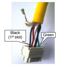
Figure 8-13: Connecting the sensor cable to sensor end connector
