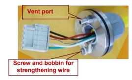
Figure 8-14: Connecting the sensor
