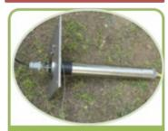
Datalogger/ Barometric Pressure Semson
