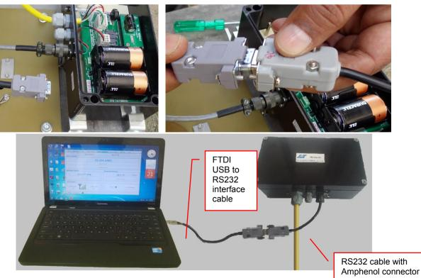
Figure 9-14: ESCL-10VT-BX Datalogger connection to Laptoph-
