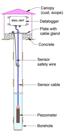
Figure 9-10: Installation of EWLR-101BX in custom made enclosure (customer scope)
