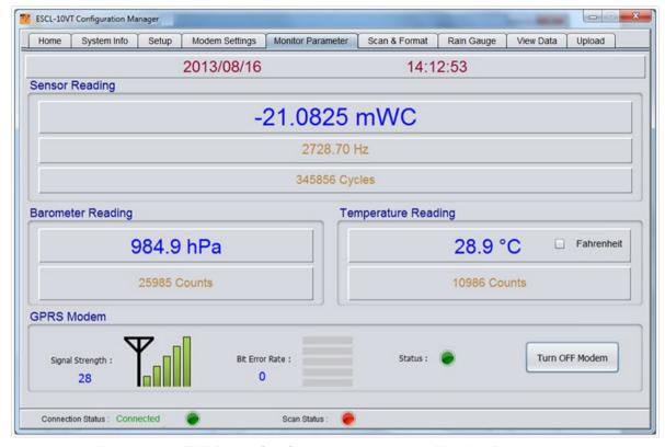
Figure 9-17: EWLR-101 Configuration manager – Monitor Parameter
