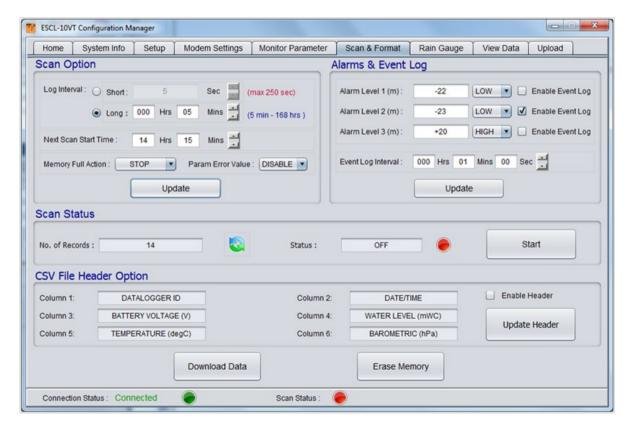
Figure 9-19: EWLR-101 Configuration manager - Scan & Format
