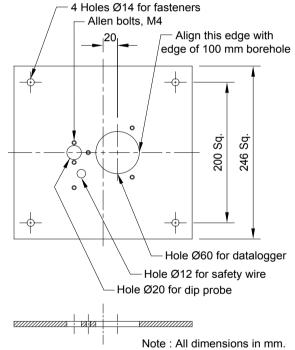
Figure 8-2: Stainless steel holding plate
