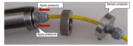
Figure 8-19: Connecting sensor end assembly to datalogger
