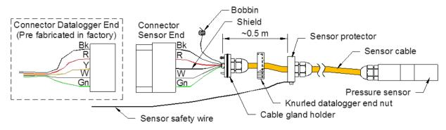
Figure 8-17: Datalogger to sensor cable wire assembly
