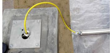
Figure 8-33: Taking out datalogger from borehole
