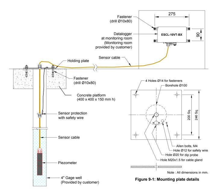
Figure 9-2 Typical installation scheme for EWLR-101BX system
