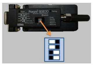
Figure 7-5: Bluetooth modem DIP switch setting
