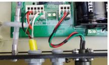
Figure 9-5: Sensor wiring to datalogger
