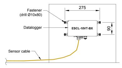
Figure 9-11: Mounting details of ESCL-10VT-BX datalogger
