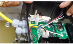
Figure 9-4: Connecting sensor cable to datalogger
