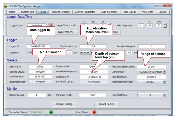
Figure 9-16: EWLR-101Configuration manager - Setup
