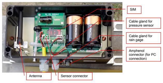
Figure 9-13: ESCL-10VT-BX Datalogger with telemetry option
