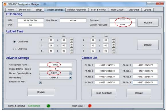
Figure 9-18: EWLR-10 Configuration manager - Modem setting
