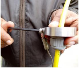
Figure 9-3: Fixing sensor protector
