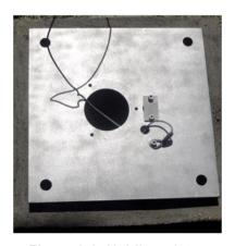
Figure 8-6: Holding plate fixed with sensor safety wire
