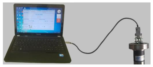
Figure 7-3: Connecting datalogger using interface cable
