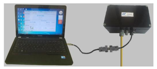
Figure 7-4: Connecting datalogger using interface cable
