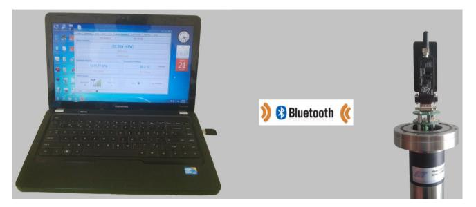
Figure 7-6: Connecting datalogger using Bluetooth
