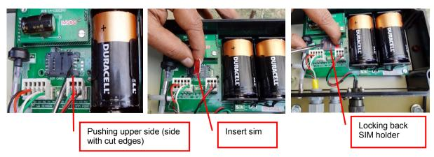
Figure 9-12: Inserting SIM
