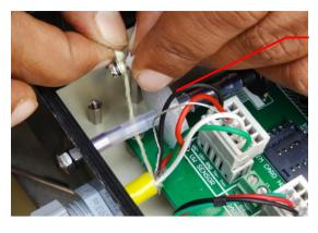
kevlar reinforce ment being fastened to the bobbin/ screw assembly
