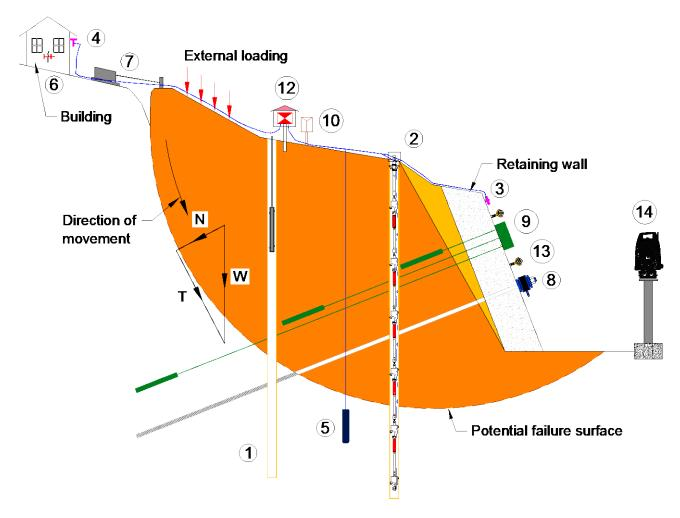
Figure 1: Field instrumentation for landslide monitoring
