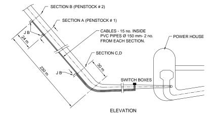
Figure 2. In the particular project, instrumentation was done in three sections (about 7 m dia) spread over a distance of 230 m
