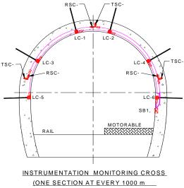
ABBREVATION LC ROCK BOLT LOAD CELL, RSC SHOTCRETE / CONCRETE STRESS CELL - RADIAL, TSC SHOTCRETE / CONCRETE STRESS CELL - TANGENTIAL,
