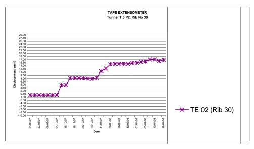
Figure 8B. Data obtained from Tape Extensioneters at the same place. Immediate corrective actions were taken following this abnormal convergence.
