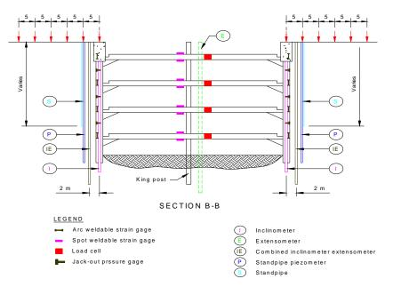
Figure 10. Typical cut and cover station box monitoring section. The distances are those used in this particular site and may vary for others depending upon specific site conditions
